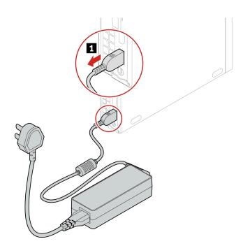
2. Disconnect the power cord from the ac power adapter.
