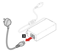
3. Push the ac power adapter out of the power adapter bracket. Remove the ac power adapter.
